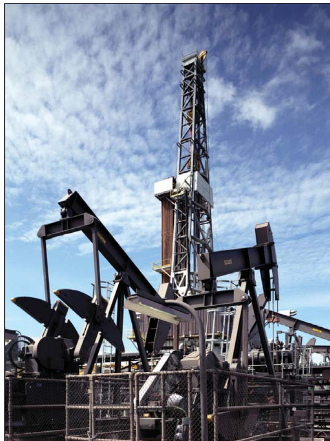
Pumping units in Wytch Farm field have close spacing that may interfere with line-of-sight communications. Photo from BP.
